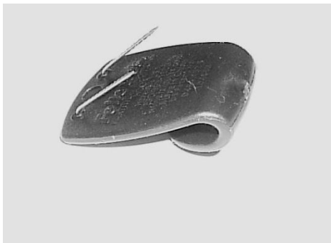
Photo B: (plastic hook provided for VetteCargoNets™ attach points) Keep steel pins aligned parallel to each other and not bent or crooked before inserting into carpet.
